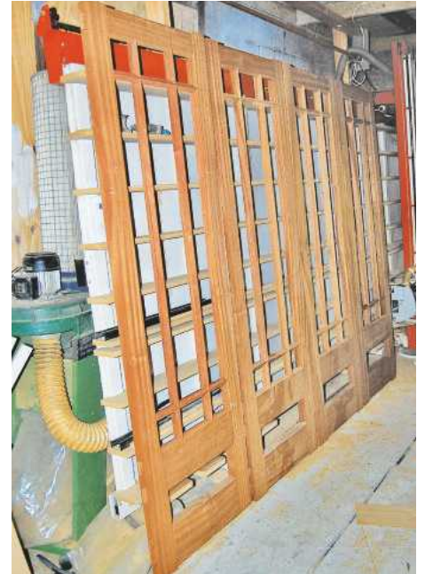
▲ Pic.20 The dry fit proved to be successful, calling for only minor adjustments
